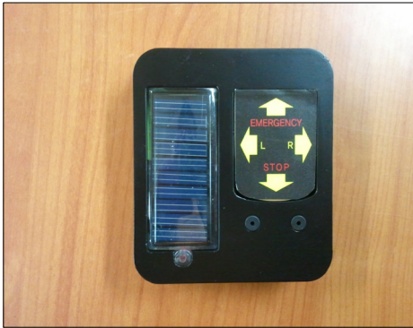
[Fig. 4] Turn signal system layout powered by solar cell
