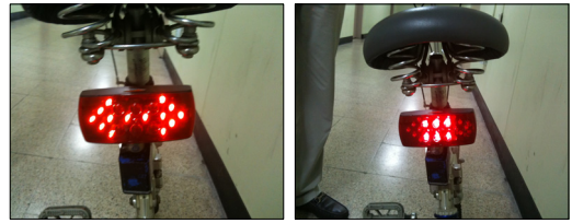
[Fig. 6] Emergency signal(left), stop signal(right)
