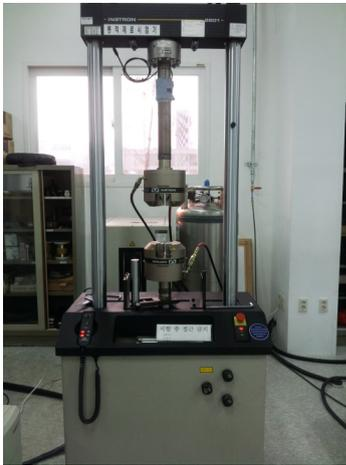
[Fig. 3] Hydraulic testing machine
