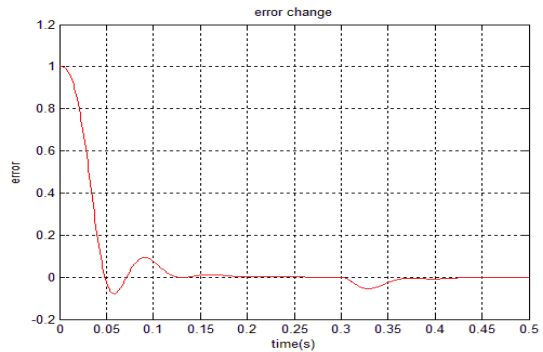
[Fig. 16] error change of PID control
