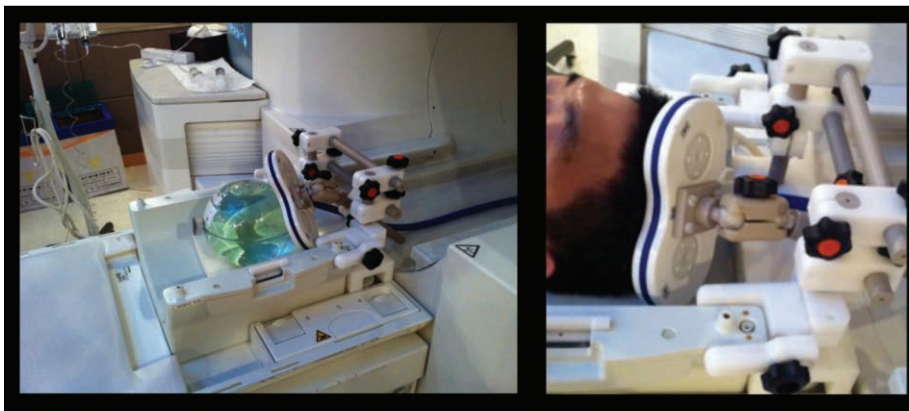
Fig. 4. (a) MR compatible coil holder setup and (b) neuronavigation system. a. MR-compatible holder setup for the MR phantom and healthy subject tasks. b. Neuronavigator (Brainsight2) guides the motor region. Activation map obtained from a simple motor task was overlaid on top of the individual's own structural image.
