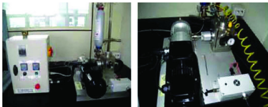
Fig. 1 Modified TE90 lubricity tester for pressurized DME fuel
