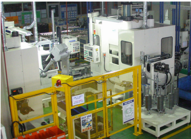
Fig. 8 The pulley forming system testbed in KAPEC company
