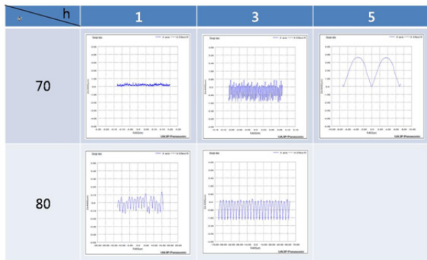
Fig. 9 Profile measurement on 70° and 80° patterns
