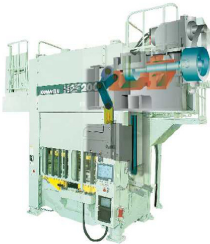
Fig. 1 Servo motor driven press system
