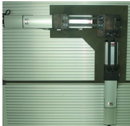
Fig. 2 Prototype 2-PPa TPM with linear actuation
