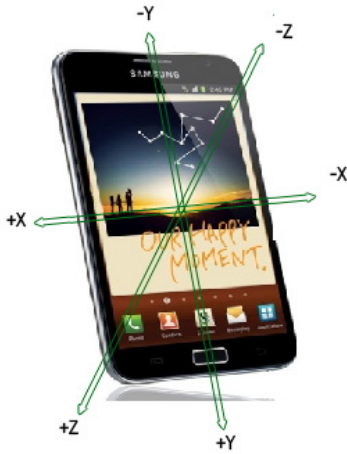
[Fig. 1] The local coordinate system of a smartphone
