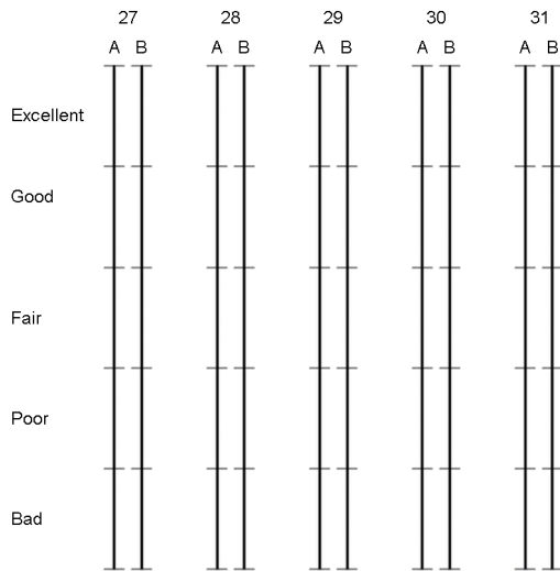
Figure 3. Evaluation scale of DSCQS (ITU-R BT.500)
