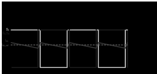
Fig. 3 Switch states and injected current waveform
