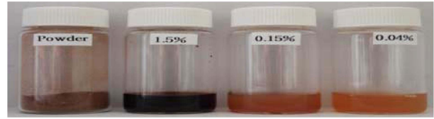
Fig. 1. Photos of pine bark powder and 1.5%, 0.15%, 0.04% solid contents of 80% methanol extracts from pine bark.
