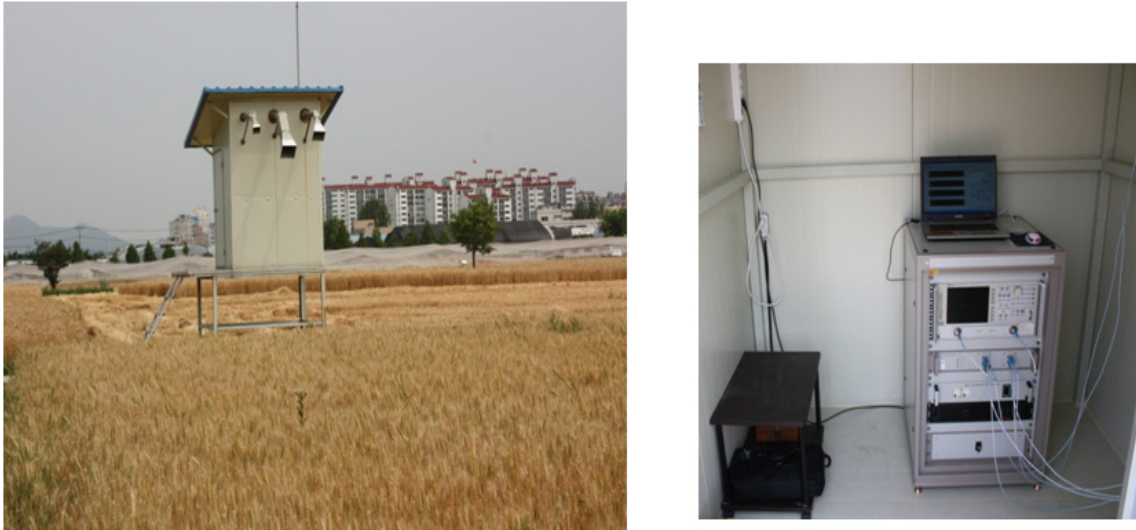
Fig. 2. Field view automatic radar scatterometer system ; (left) The shelter installed in the experimental wheat upland with an L, C, X-band looking at the 40 degree ; (right) RF systems inside the shelter with network analyzer, RF cable, RF switch and a computer that controls frequency, polarization and data storage.
