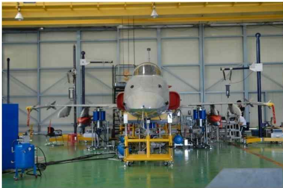
Fig. 3. Ground Vibration Test of Whole Aircraft(F-5)
