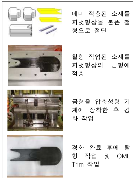
Fig. 4. Compression molding procedure
