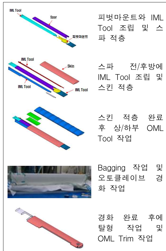
Fig. 5. Autoclave molding procedure
