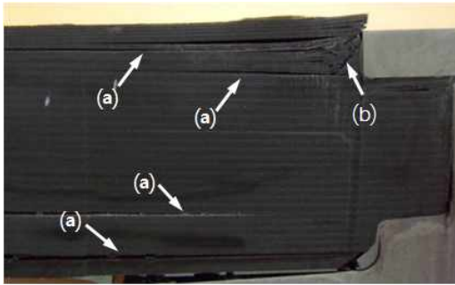
Fig. 20. Section photo of specimen(b) : delamination(a), fiber broken(b)
