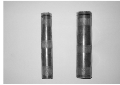
Fig. 6. Frozen SCP for sand-clay composite soil
