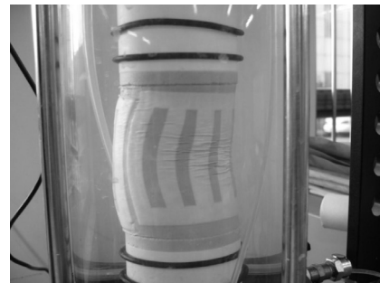
Fig. 12. Buckling failure of sand-pack-clay composite soil
