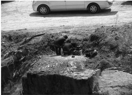
Fig. 2. Installation of accelerometer on the outcropping rock
