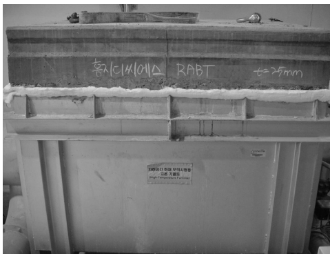
Fig. 7. Test specimen on a heating device
