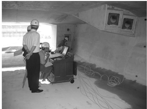
Fig. 3. View of the impact test conducted in the 50m PSC box-girder
