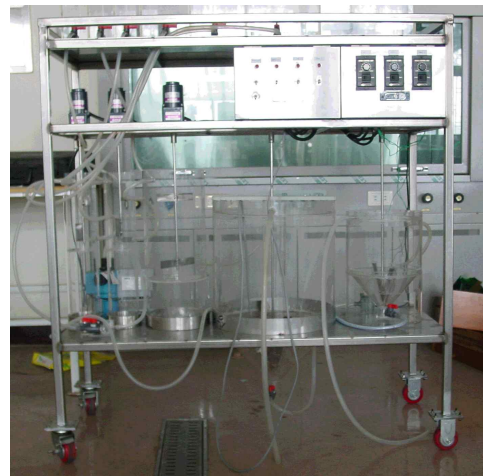
Photo. 1. Photograph of pilot plant on copper removal.
