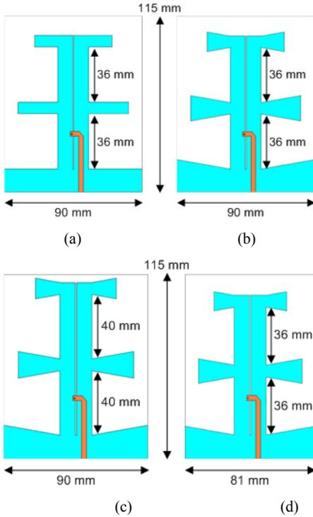
[Fig. 2] Design procedure of proposed SBDP antenna.
