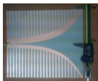
(b) 제안한 비대칭 corrugated TSA (b) Proposed TSA with asymmetric corrugation
