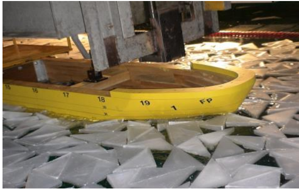
Fig. 7 Profile of resistance test with synthetic ice.
