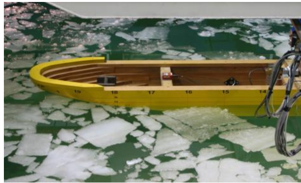
Fig. 9 Profile of resistance test with refrigerated ice.
