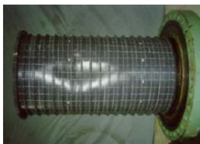
Fig. 2 Model failed by inelastic overall collapse.
