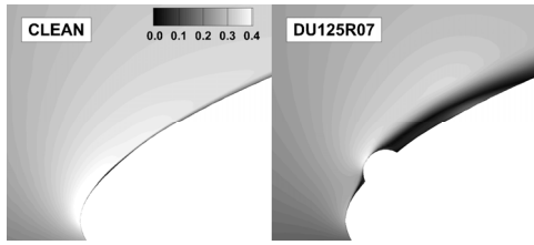
Fig. 6 Velocity distribution change due to contaminant accumulation (angle of attack: 9.22°)
