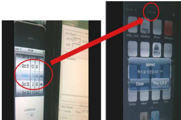
Fig. 12 Alarm operation using Local Notification function
