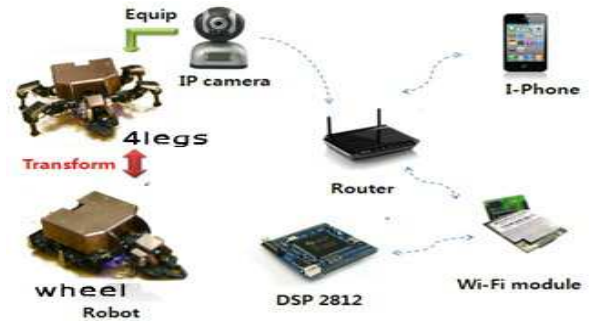
Fig.2 Robot system structure
