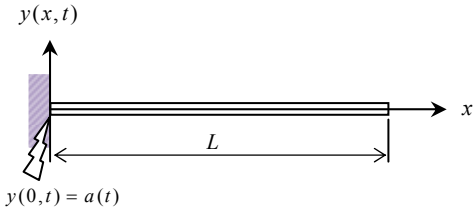
Fig. 3 Cantilever subjected to a support motion
