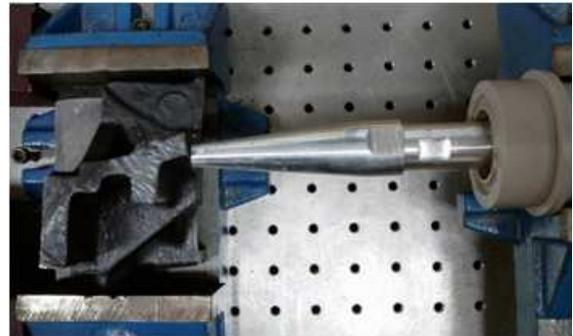
Fig. 6 Fixed to press into specimen and horns
