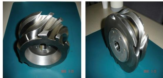
Fig. 8 Shape of designed cylindrical cam
