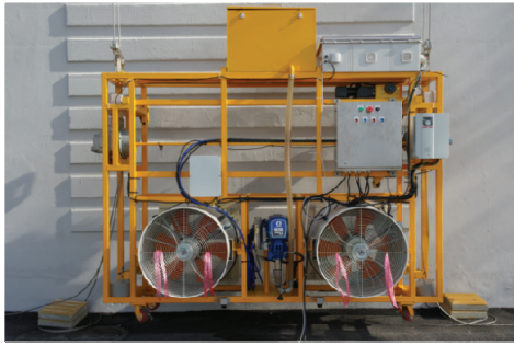
Fig. 1 Gondola-typed Façade Robot
