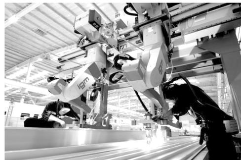
Fig. 3 Gantry system for MIG welding
