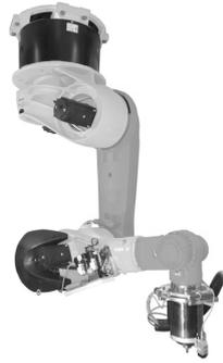
**Fig. 6** Robot for FSW(attached with welding head and sensors)
