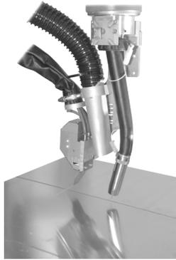
**Fig. 4** Laser camera sensor for weld seam tracking (iCAM)
