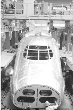
Fig. 1 Welding robot system for high speed trains
