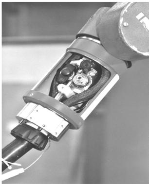
Fig. 2 Torch drive for welding wire feeding
