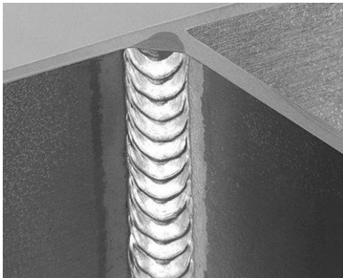
Fig. 12 Bead appearance of aluminium weldment by using synchro-pulse program
