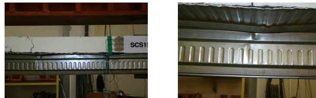
(a) Loading point crack (b) Local buckling Fig. 5 Fracture mode of specimens (SCS150-1.0N)
