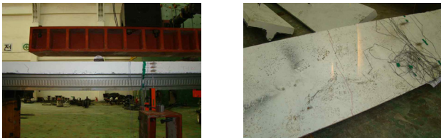
(a) Loading point crack (b) Topping Crack Fig. 7 Fracture mode of specimens (SCS200-1.0N)
