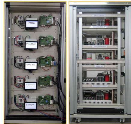
Fig. 8. Structure of DC Micro-grid Assembly.
