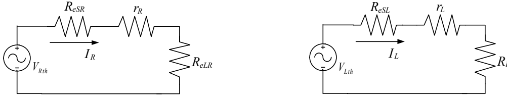
(c) Equivalently simplified circuit transformed to the receiver coil. (d) Equivalently simplified circuit transformed to the load coil.
