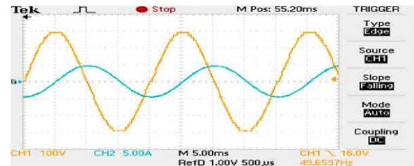
Fig. 10. Experimental results of total output voltage and output current for the inductive load.
