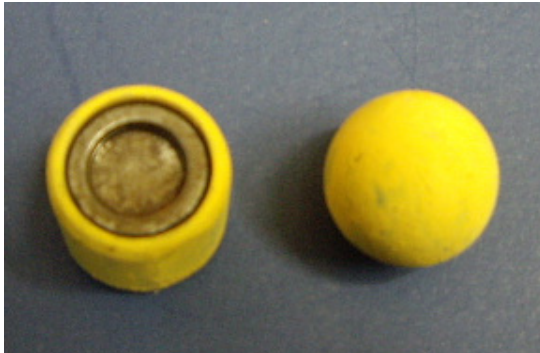
Fig. 12 Wear of ball and roller
