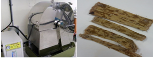
Fig. 1. Drum-type rotary debarker (left) and primarily debarked mulberry bast part (right).
