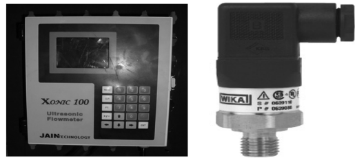
a)Ultrasonic flowmeter b)pressure sensor
