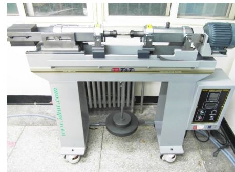
Fig. 2 Rotary bending fatigue tester
