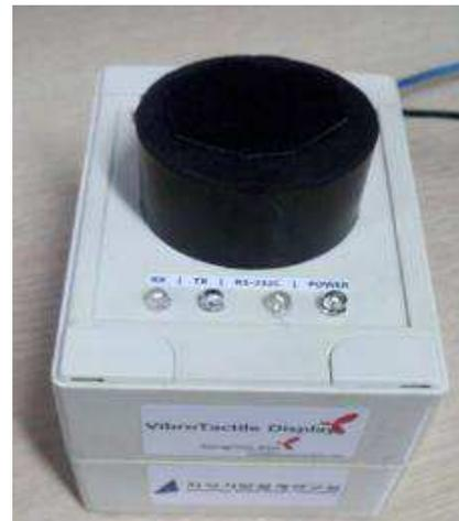
Fig. 7 Vibro-Tactile display device
