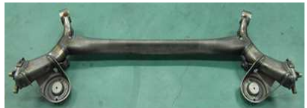
Fig. 8 Prototype of tubular torsion beam axle
