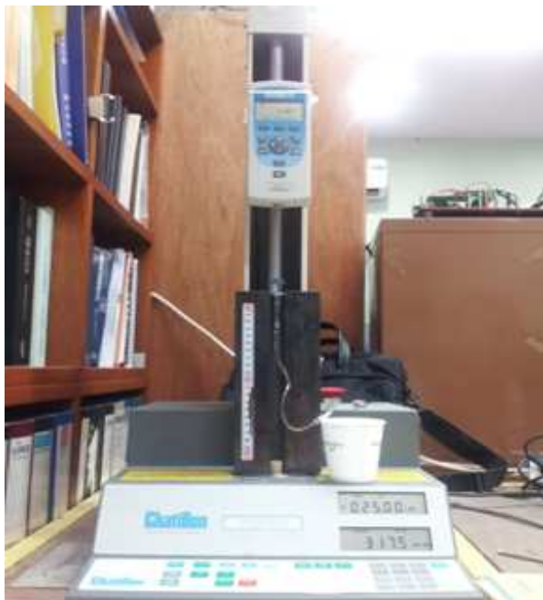
Fig. 4 Internal pressure measuring device of drug injector
