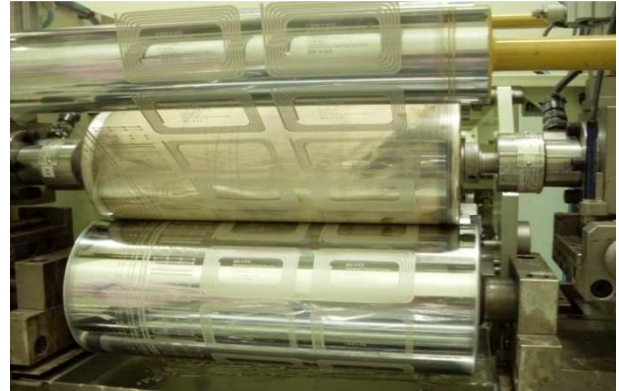
Fig. 2 Direct gravure printing equipment
