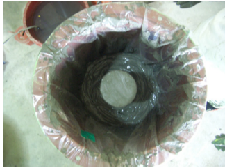
[Fig. 4] Preparation of clay layer
