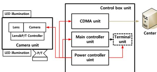
[Fig. 1] Composition of image stage gauge system
