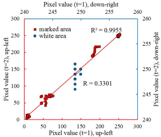
[Fig. 6] Correlation characteristic by inspection area position
