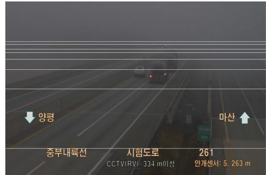
[Fig. 6] An example of the still images stored in 5 minutes once (Oct. 26, 2012, 07:19:12 RVMS measurement result: 334m, fog sensor measurement result: 5,263 m) and the sidelines (50, 100, 150, 200, 250, 300, 400, 500m)
