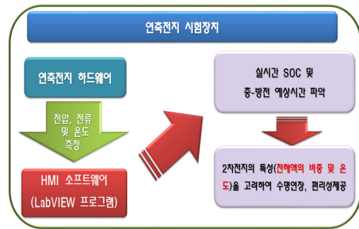
[Fig. 4] Concept of SOC test device of lead-acid battery
