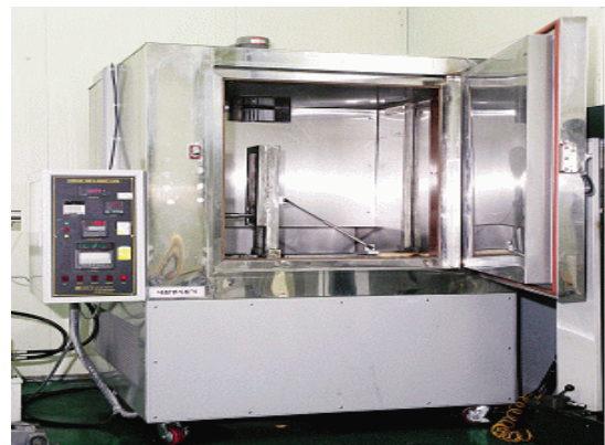
Fig. 7 Photo of salt water tester chamber
