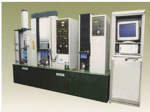
Fig. 5 Photo of compression test and durability test (Test stroke : 170mm), (Test speed : 2 mm/sec)
